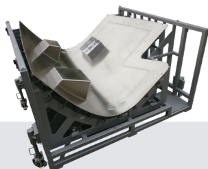
A320 Belly Fairing Made for AIDC
