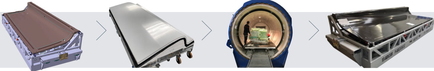
Autoclave dimensions: Ø 3 m - L 10 m - 250° C - 10 bar
