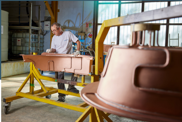
Copper part for particle accelerator Dimensions: 1200*1100*350 mm Weight: 70 Kg Deposit: copper up to 10 mm on some areas.
