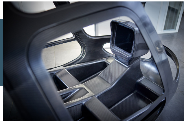
ULM helicopter cabin. Composite part, hollow body with internal and external skin.
